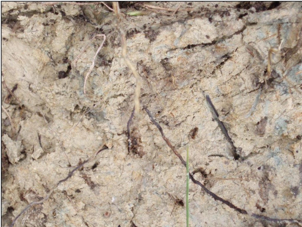
Photo 10: Clay soils with gleying and redoximorphic features in Wetland 5.
